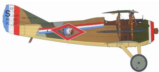
1917 SPAD S.13 100 hp Hispano-Suiza 8B 8-cylinder water-cooled Vee engine Span 30 ft 6 in, length 26 ft 6 in, height 10 ft 6 in; maximum speed 130 mph at 5,000 ft; climb to 6,000 ft in 10 min 40 sec; ceiling 21,000 ft; empty weight 1,200 lb; loaded weight 1,800 lb Armament: one fixed synchronized Vickers machine gun
