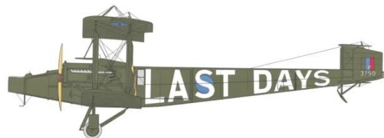
1918 HANDLEY PAGE O/400 Two 100 hp Rolls-Royce Eagle VIII 12-cylinder water-cooled Vee engine Span 100 ft, length 60 ft 6 in, height 20 ft; maximum speed 117 mph at sea level; climb to 6,000 ft in 27 min 40 sec; service ceiling 6,000 ft; empty weight 6,500 lb; loaded weight 12,000 lb Armament: four 7.92 mm fixed-mounted Lewis machine guns in nose, wings, and belly positions; typical bomb load carries 120 lb bombs
