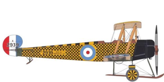
1917 AVRO 504K 110 hp Le Rhône 9-cylinder air-cooled rotary engine Span 34 ft, length 28 ft 6 in, height 10 ft 6 in; maximum speed 110 mph at sea level; climb to 6,000 ft in 16 min; service ceiling 16,000 ft; empty weight 1,200 lb; loaded weight 1,800 lb
