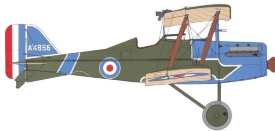
1917 S.E.5 130 hp Hispano-Suiza 8-cylinder water-cooled Vee engine Span 30 ft 10 in, length 25 ft 6 in, height 8 ft 6 in; maximum speed 135 mph at 6,000 ft; climb to 6,000 ft in 8 min; service ceiling 17,000 ft; empty weight 1,200 lb; loaded weight 1,800 lb Armament: one fixed synchronized Vickers machine gun; one Lewis machine gun mounted over top wing
